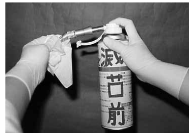
図6 滅菌前オイルの注入 fig. 6 Injection of pre-sterilization oil
